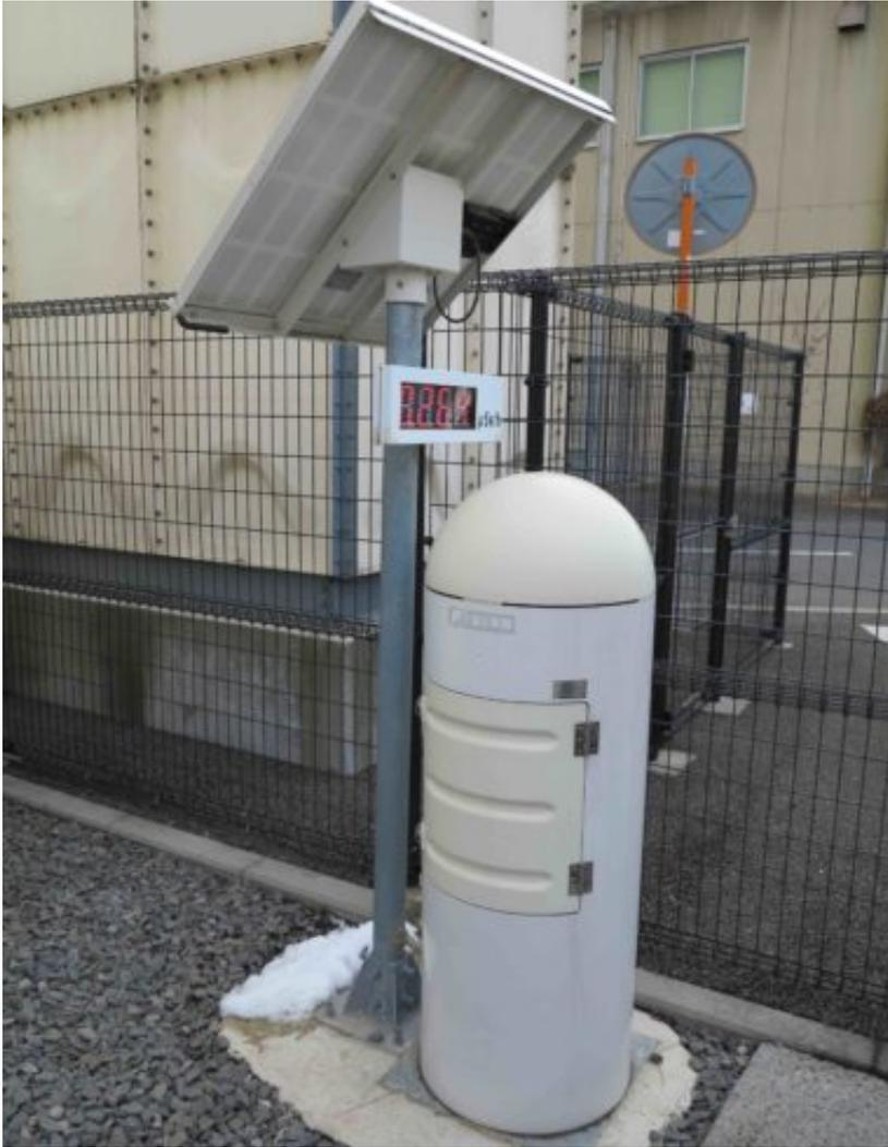
Numerous radiation monitoring posts were installed in Fukushima prefecture. Photo by the author
